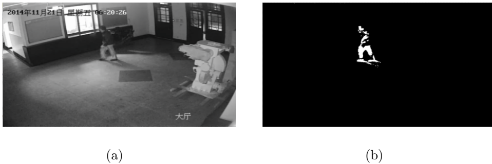
FIGURE 4. Original image in the video and the image of the foreground extraction
