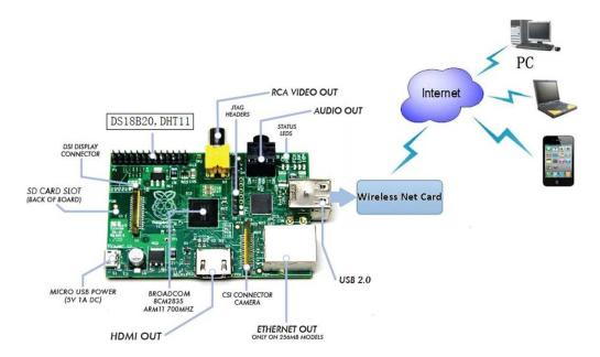
FIGURE 1. Overall system structure with different sensing units
