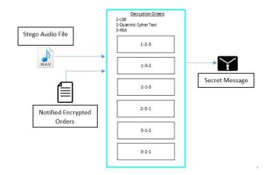
FIGURE 2. Data decryption (receiver side)
