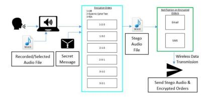
FIGURE 1. Data encryption system (sender side)
