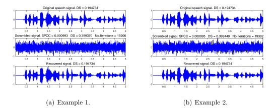
FIGURE 3. Examples of two scrambled signals from the same original speech signal.
