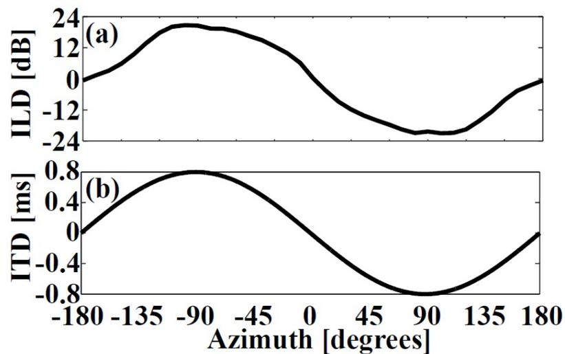
FIGURE 3. Interaural difference (a) the mean of the measured ILDs, (b) ITD model of sphere
