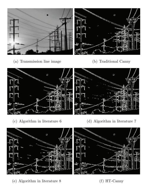
FIGURE 7. Edge detection results of Transmission Line image
