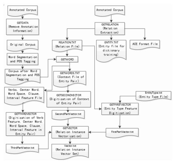
FIGURE 3. Entity relation instance vectorization program flow chart
