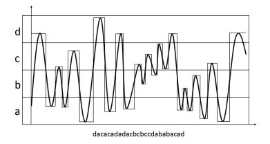
FIGURE 3. Signal partition by using SAX method
