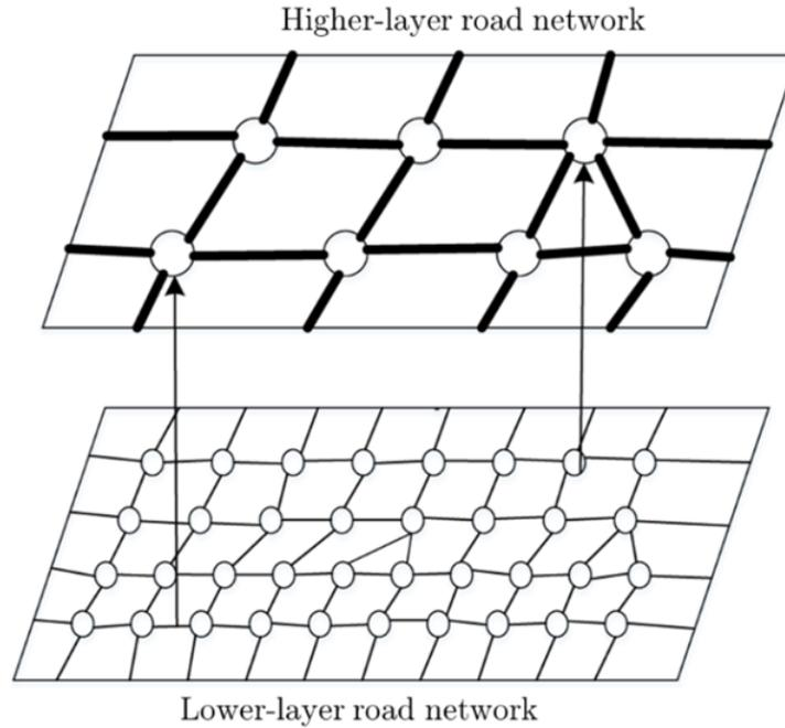
FIGURE 2. Two-layer example of road network abstraction
