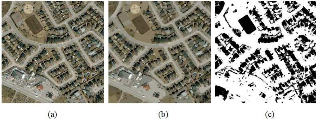
FIGURE 2. (a) Original image. (b) The clustering result by our mean shift method. (c) Result of detecting road regions from Fig. 2(b) by traditional threshold method.
