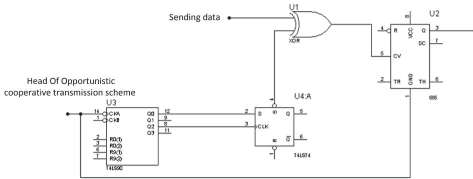
FIGURE 12. Implementation of circuit signal modulation
