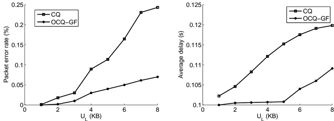
FIGURE 14. Performance with CQ and OCQ-GF. (a) Packet error rate,(b) Average delay.
