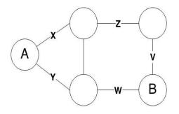
FIGURE 1. The vertices A and B in this network have more than one minimum edge cut sets, such as  $\{X,Y\}$ ,  $\{W,Z\}$  and  $\{V,W\}$ .
