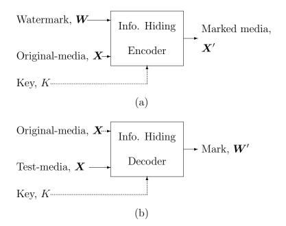
FIGURE 2. The block diagrams for information hiding [1, 2]. (a) Information insertion. (b) Information extraction.
