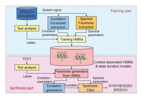
FIGURE 1. An overview of the basic HMM-based speech synthesis system [5]
