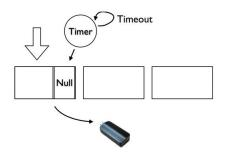
FIGURE 11. The fast transmission mechanism of send buffer on TX
