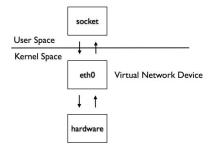
FIGURE 9. Virtual network device
