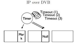
FIGURE 12. The delay padding mechanism of send buffer on TX
