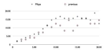
FIGURE 15. Data rate of polling mechanism with idle checking on RX ring buffer (X axis: seconds, Y axis: Mbps)
