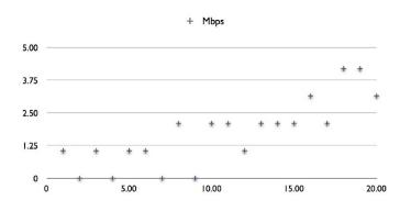
FIGURE 13. Effcient data rate of TX with rough null data padding (i.e., fast transmission padding mechanism) (X axis: seconds, Y axis: Mbps)
