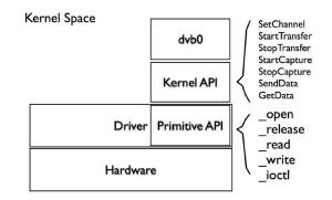
FIGURE 10. Modified architecture of driver
