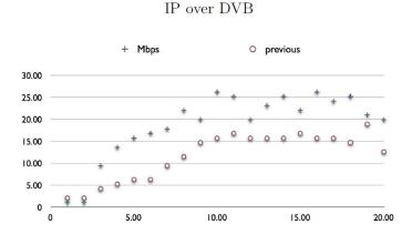
FIGURE 16. TCP throughput over DVB network (X axis: seconds, Y axis: TCP throughput in Mbps)
