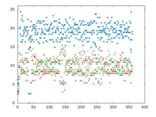
FIGURE 21. Throughput of two TCP connections (X axis: seconds, Y axis: Mbps)
