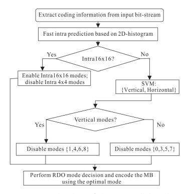
FIGURE 6. Flowchart of the proposed algorithm
