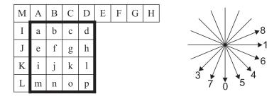
FIGURE 1. Pixels used in intra  $4 \times 4$  and the prediction directions.
