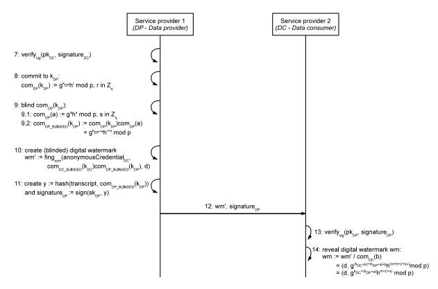
FIGURE 3. Phases B and C of the DETECTIVE Tag protocol.
