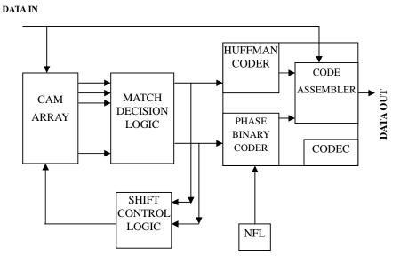
FIGURE 3. Compressor Coder Internal Block Diagram.
