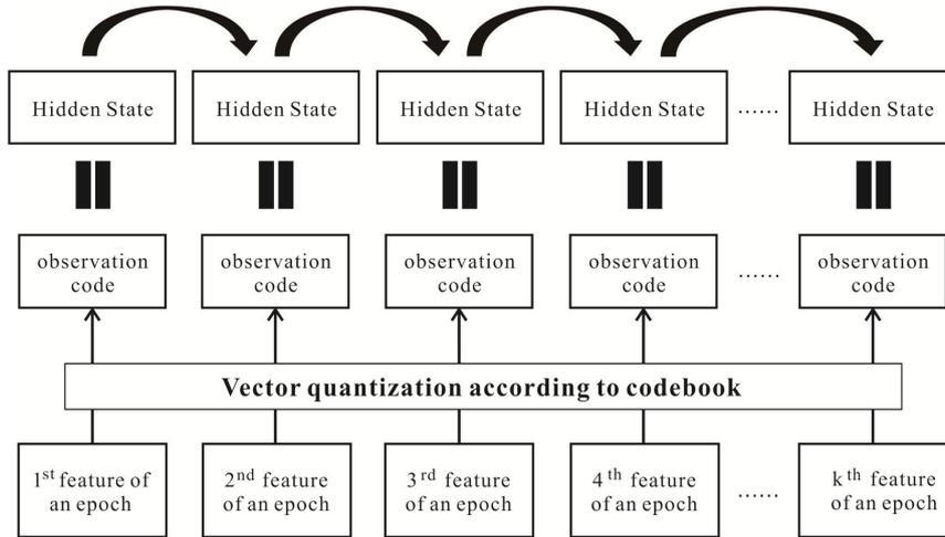
FIGURE 3. Relation between the features of speech, the observation and the hidden states of DHMM
